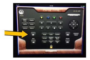
To adjust the audio volume, press "audio" at the bottom of the screen, as shown, to bring up the sound control screen. Then use the "Blu-ray" slider icon to set the sound level. This controls the amplitude of the output from the DVD player. More volume can be achieved by using the "Banquet" slider, which controls the output of the system amplifiers.
